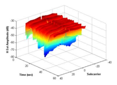
Custom experimental framework allows deep visibility into PHY. Per-packet, per-subcarrier channel estimates are shown.
